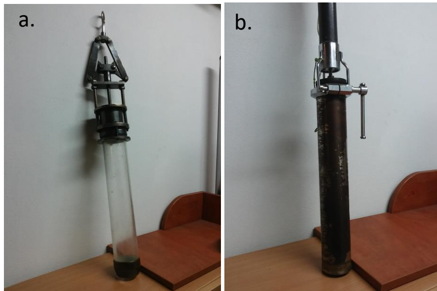
Figure 2. Pictures of the two core samplers used for the collection of samples of macroinvertebrates: (a) Kajak corer (b) Czaplą corer
