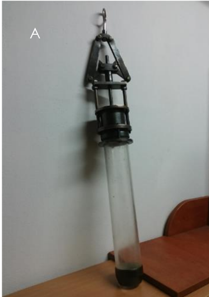
Kajak Sampler diameter 6,0 cm
