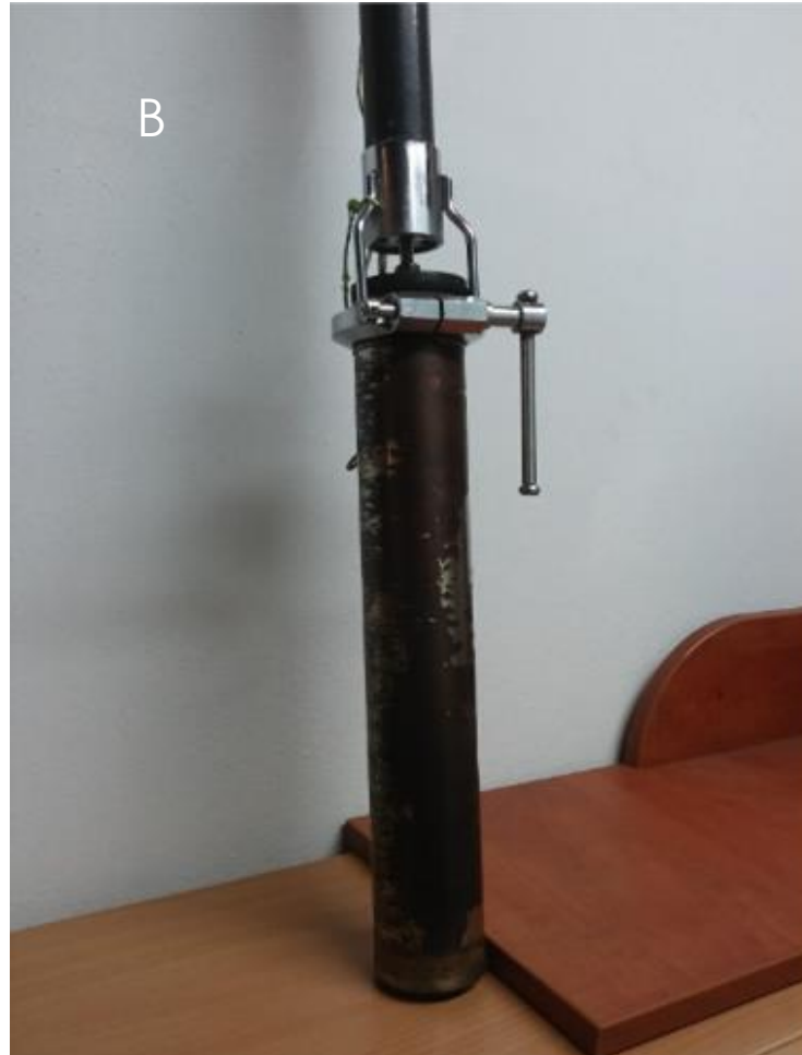
Czapla Sampler diameter 5,6 cm
