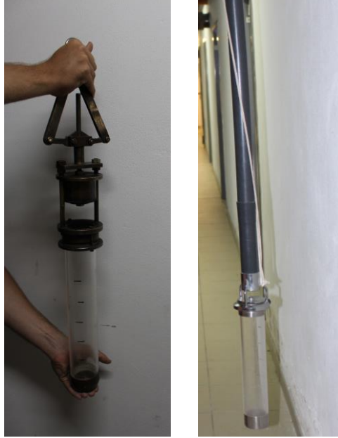
Image 2. The Kajak and Czapla samplers used to collect sediment.
